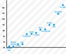
The glass transition temperature (TG) is the temperature region where the polymer transitions from a hard, glass material to a soft, rubbery material. Prints will often deform around this temperature, but it is needed for the bed to heat to just around a materials glass transition temperature in order to have good bed adhesion. You can get away with printing **PLA** on a non-heated bed, but any material with a high Tg will require a heated bed.
