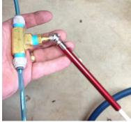
3. Push on the on the tube fitting to hold quick connect air chuck engaged and pull on the outer sleeve then in one motion pull the quick connect air chuck off of the Schrader valve. A tiny amount of air will escape and this is normal. The reason you push on the tube fitting is so you can have a consistent dismount from the Schrader valve. The following photos show the quick disconnect fitting extended and retracted. Notice you can see the lock ring when it is retracted.
