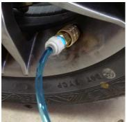
2. Remove the protective cap from the Schrader valve on the Tee and using an air gauge check the pressure and adjust the pressure as needed using any air source up to 100 psig. When you're finished both tires will have the exact same pressure.
